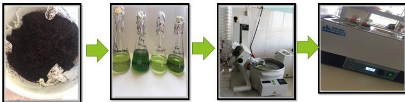
Figure 2. The extraction steps of U.rigida
