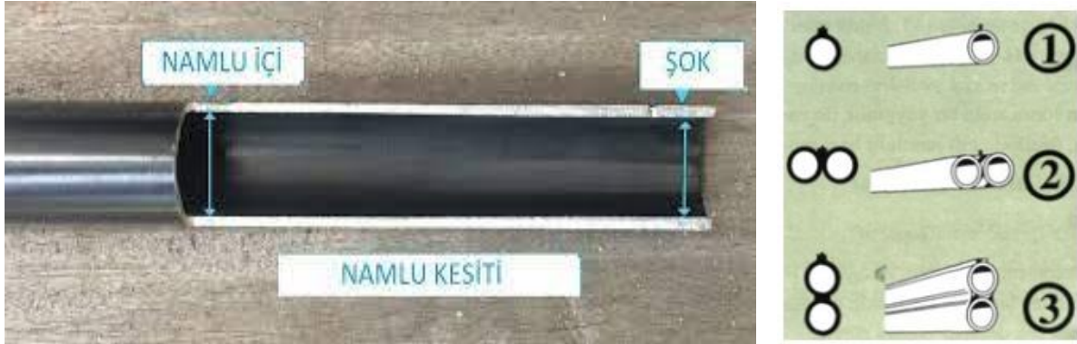
Figure 2. Detailed views of the smooth barrel [6]; a) sectional view, b) various barrel structures.
